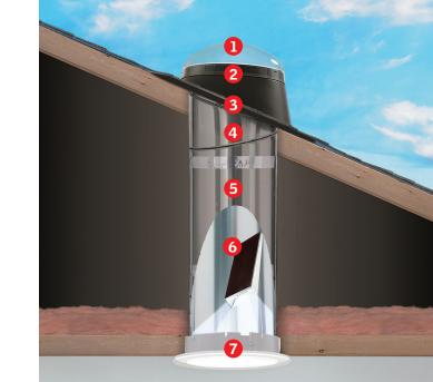
VELUX Sun Tunnel skylights fit between ceiling beams, allowing sunlight to travel from the roof to the space below uninhibited.
