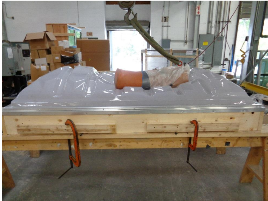
Photo No. 2 Test Specimen with 400 lb. Weight Applied
