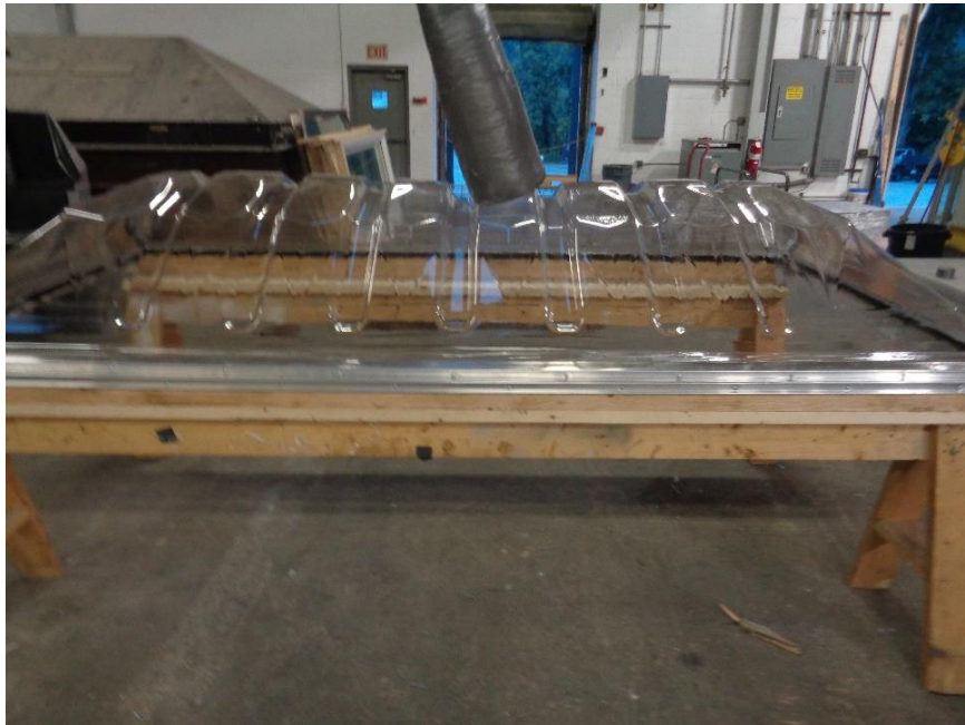
Photo No. 2 Test Specimen during 400 lb. Load
