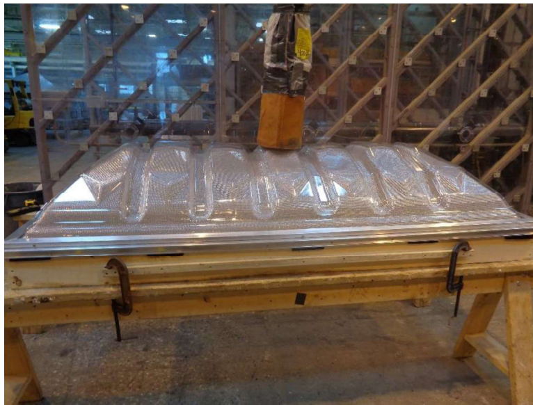
Photo No. 2 View of Tested Specimen with 400 lbs Applied
