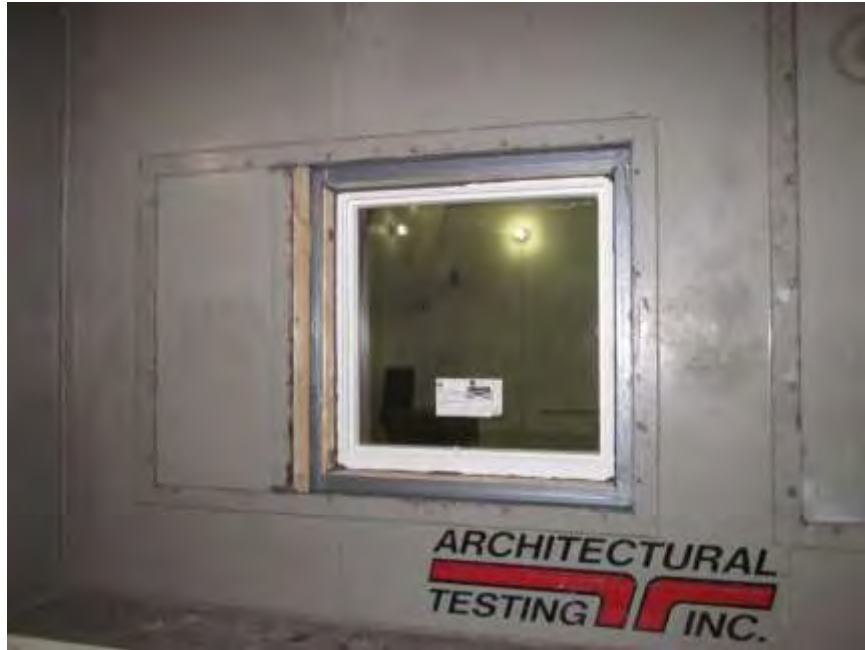
Receive Room View of Installed Specimen
