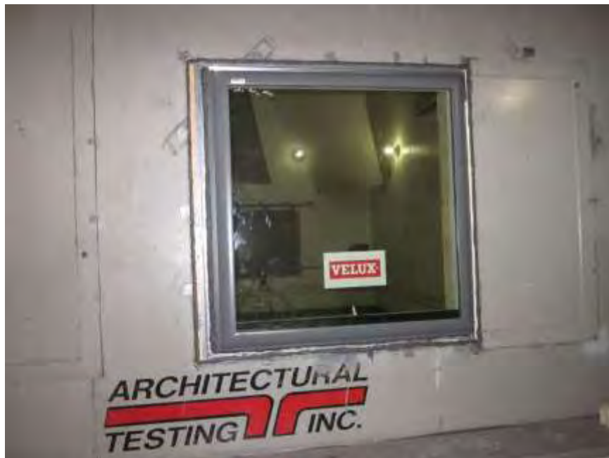
Source Room View of Installed Specimen
