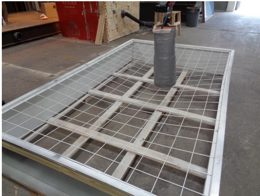
Photo No. 2 Test Specimen During 400 lb. Load
