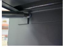
Remove screws securing VCS to curb and rest VCS on curb as shown.
