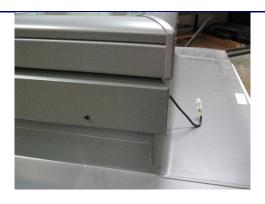
Place the solar panel at the top of the VCS with the top of the panel level with the top of the stationary frame and centered as shown.
