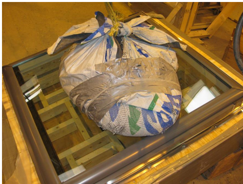
Photo No. 2 Test Set-up and 200 lbf Bag
