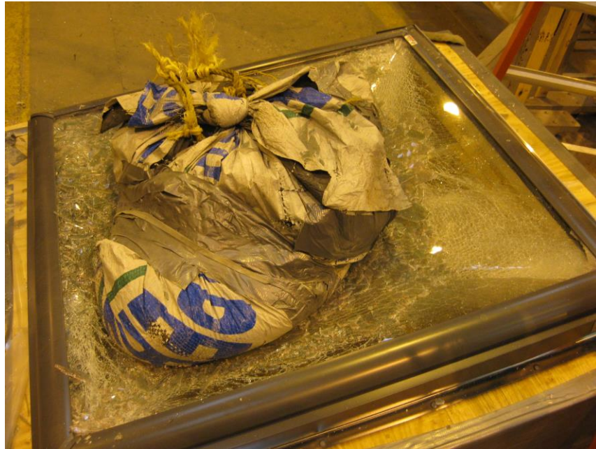
Photo No. 3 Result from 10' Drop Height
