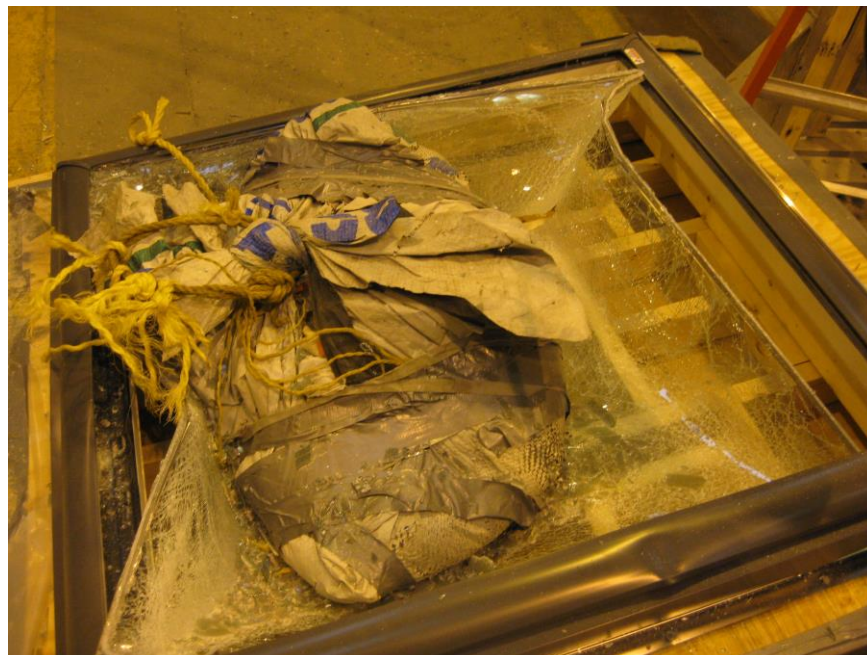
Photo No. 4 Result from 12' Drop Height
