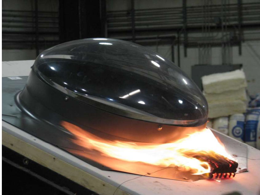
Photo No. 4 Burning Brand #1 Placement (During Test)
