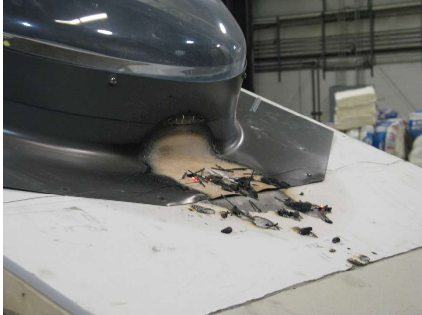
Photo No. 6 Extent of Damage After Brand #1
