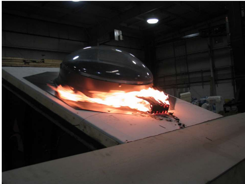
Photo No. 7 Burning Brand #2 (During Test)
