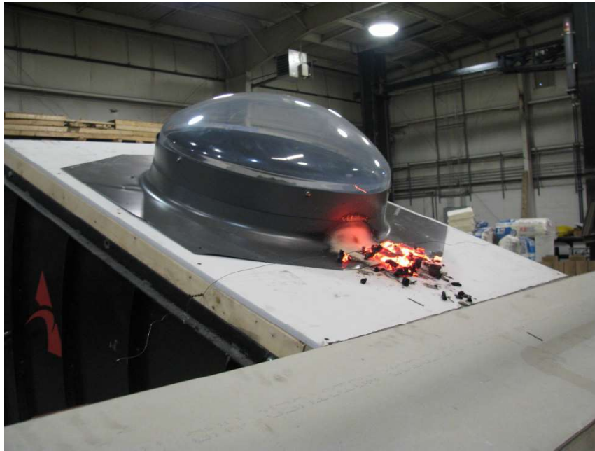
Photo No. 9 Extent of Damage After Brand #2
