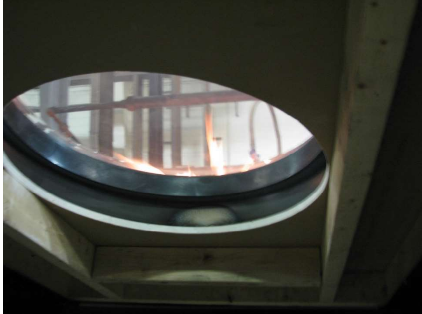
Photo No. 8 Underside of Deck During Brand #2 Exposure
