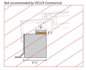
Steel, concrete or wood construction with wooden batten
