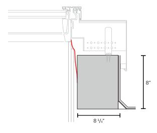
The sub-construction can be finished at the bottom with steel profile, which provides a level and stable surface for the skylight modules and forms a base for fitting mounting brackets with clamps.
