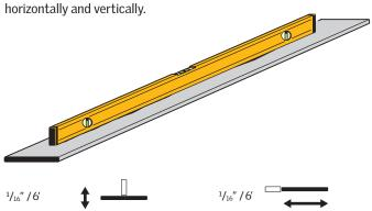
The following standard flat steel profiles are suited for installation of VELUX modular skylights in Ridgelight solutions.
