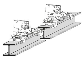
Connection of steel profiles must not collide with clamps
