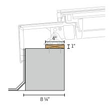
Steel, concrete or wood construction with wooden batten
