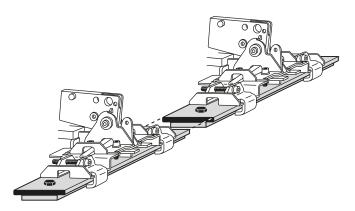
• Connection of flat steel profiles must not collide with clamps
