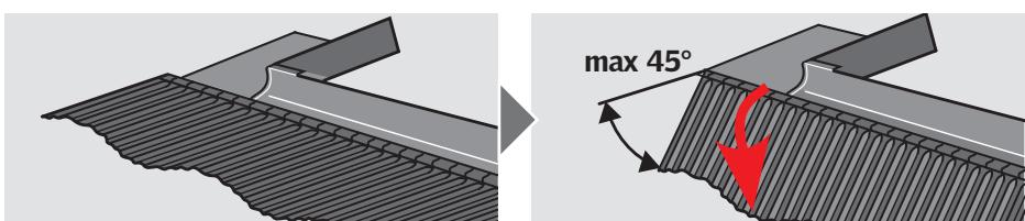
**ENGLISH:** Reposition sill flashing section and attach it to curb with roofing nails as shown.
