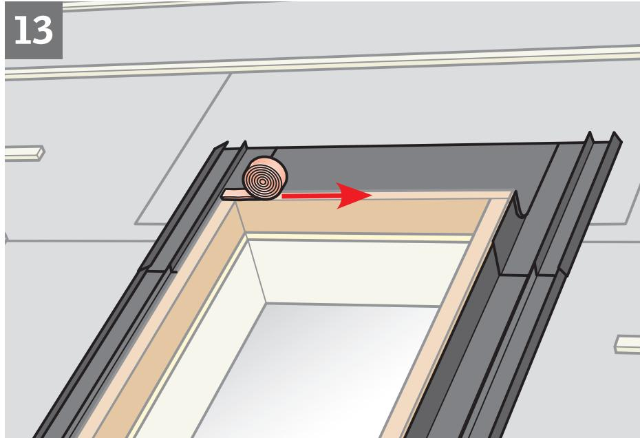
**ENGLISH:** To prevent condensation, application of foam gasket (not provided by the manufacturer) is recommended at the top of the curb before attaching counter flashing.
