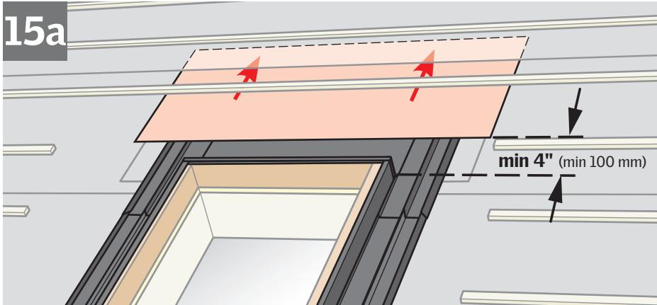
**ENGLISH:** To allow for proper drainage, interweave roofing underlayment as shown in **15a** for new construction applications. For retrofit applications, interweave roofing underlayment as shown in **15b**.
