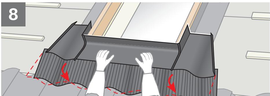
**ENGLISH:** Remove sill flashing section and bend the apron down as shown. This will ensure that the apron lies tightly against the roofing material.
