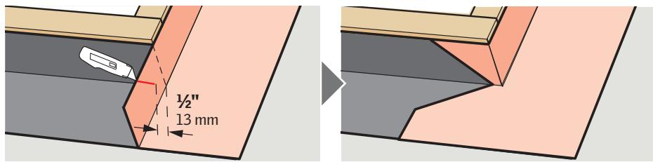
**ENGLISH:** Wrap the bottom and the corners of the skylight curb with VELUX adhesive skylight underlayment and create watershedding laps over roofing underlayment.
