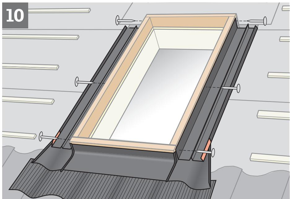
**ENGLISH:** Cut side sections to match size of curb. Modify side sections to allow for a smooth transition from sill flashing section to deck level and attach side sections to curb with roofing nails.
