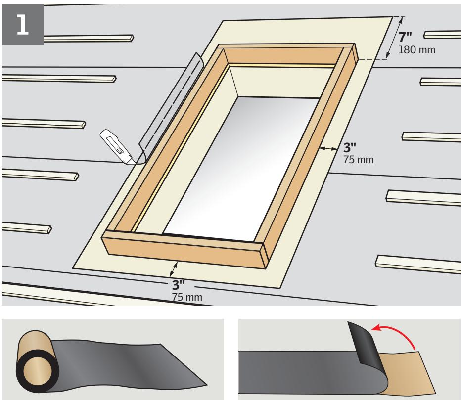
**ENGLISH:** To ensure waterproofing, skylight curbs shall be completely wrapped in VELUX adhesive skylight underlayment as indicated. Adhesive skylight underlayment must be applied before installing the flashing. Remove existing roofing underlayment around the rough opening as shown.
