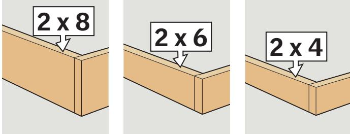
**ENGLISH:** Site-built curb to be provided by installer, with a height of 7 $\frac{1}{4}$ " (185 mm), 5 $\frac{1}{2}$ " (140 mm) or 3 $\frac{1}{2}$ " (90 mm).
