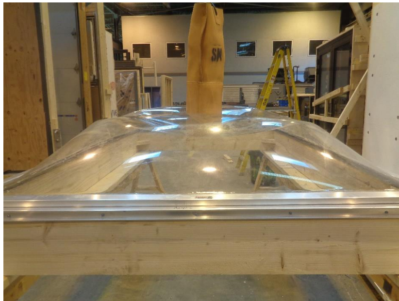
Photo No. 2 Tested Specimen with 400 lb. Load Applied
