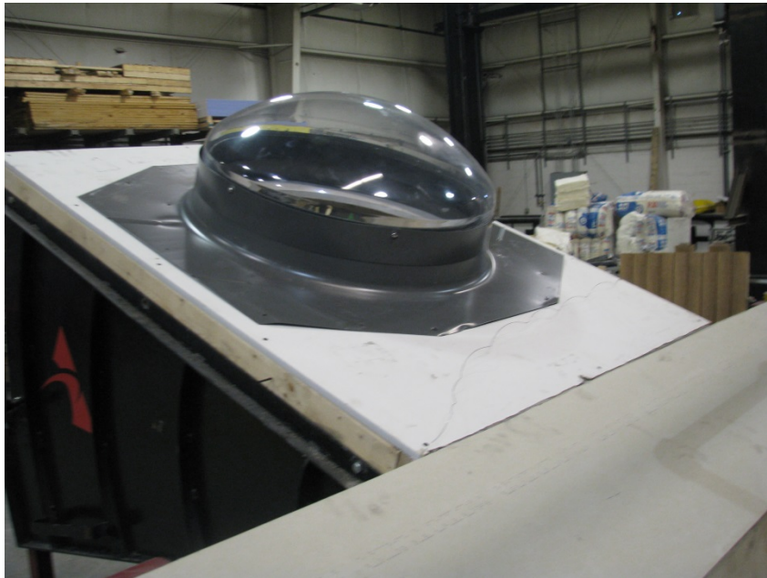
Photo No. 1 TDD Mounted to Test Deck (Pre-Test)
