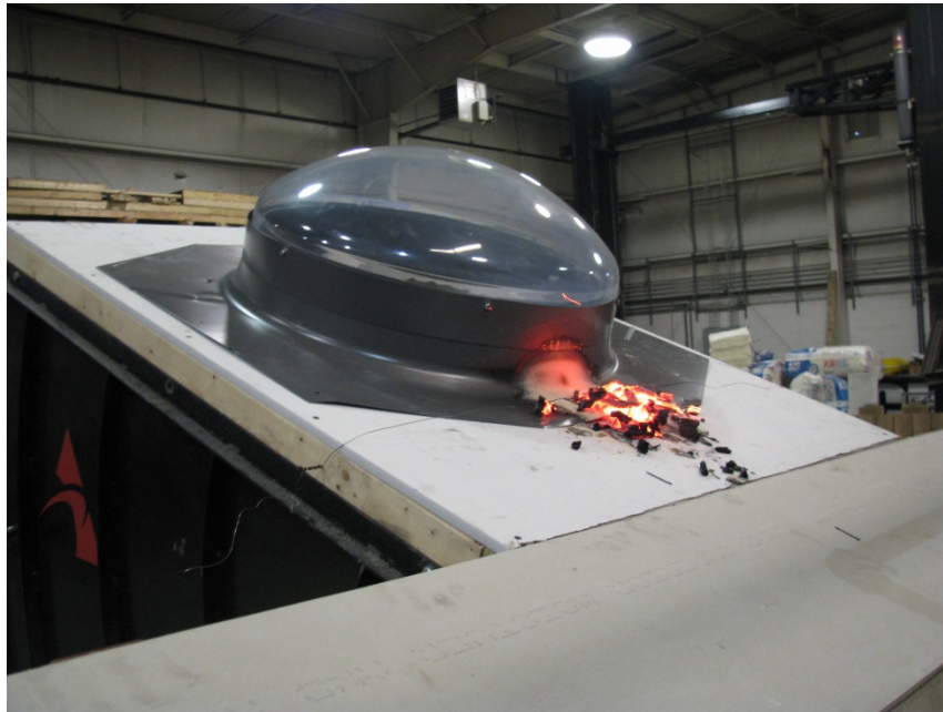
Photo No. 9 Extent of Damage After Brand #2
