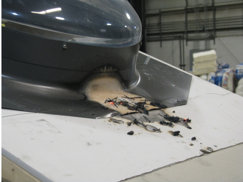
Photo No. 6 Extent of Damage After Brand #1
