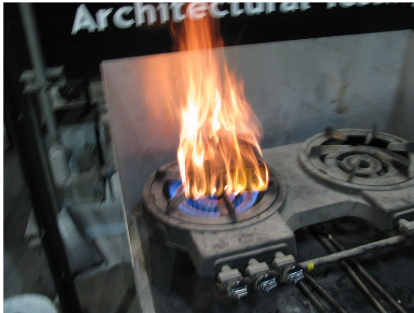
Photo No. 3 Class B Brand Ignited on Gas Burner
