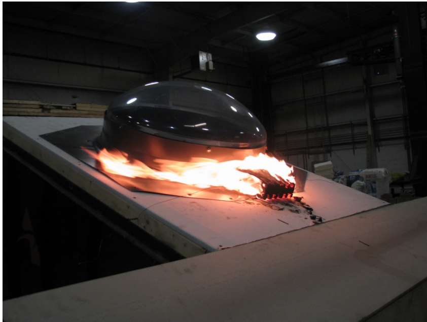
Photo No. 7 Burning Brand #2 (During Test)
