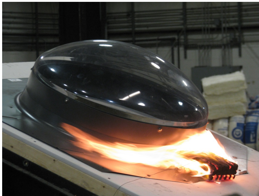
Photo No. 4 Burning Brand #1 Placement (During Test)
