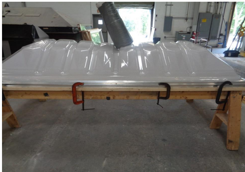
Photo No. 2 Test Specimen during 400 lb. Load
