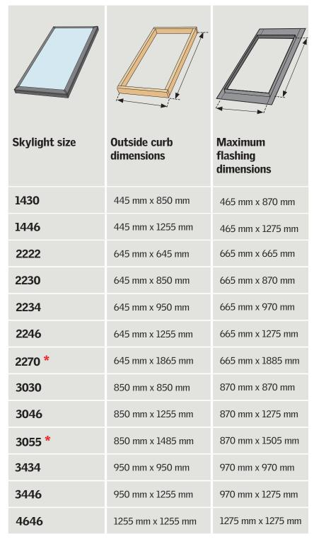
Build curb according to measurements in the chart. Use lumber with an actual thickness of 35-38 mm and a minimum height of 100 mm. Curb height and attachment should comply with building codes and regulations and be secure enough to transfer the skylight loads to the framing members.
