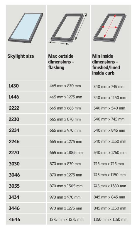
Build curb according to measurements in the chart. Curb height and attachment should comply with building codes and regulations and be secure enough to transfer the skylight loads to the framing members.
