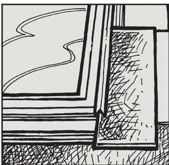
Along the side, the first layer of felt, which lies over the last course of shingles, is run under the L gasket. The first shake on the side is also positioned under the L gasket.
