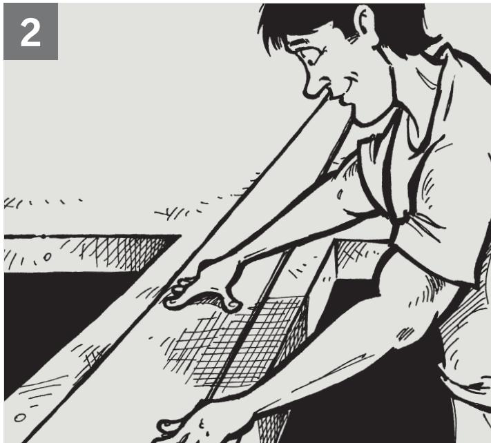
Cut two strips of Superseal 14½" longer than your rough opening height. Remove the release paper from one side of a strip of Superseal and center it between the openings over the anchor brackets you just installed. Leave the top release paper intact.
