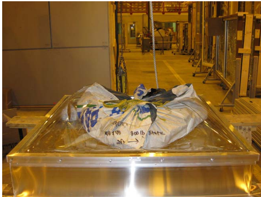
Photo No. 2 Test Specimen #1 (48 x 48) Failure
