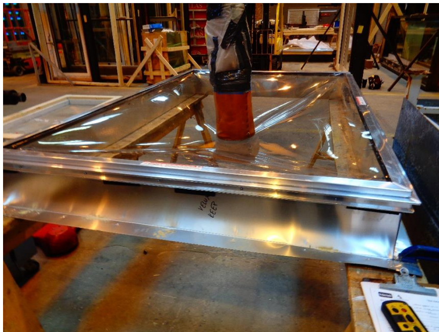
Photo No. 2 View of Tested Specimen with 400 lb Weight Applied
