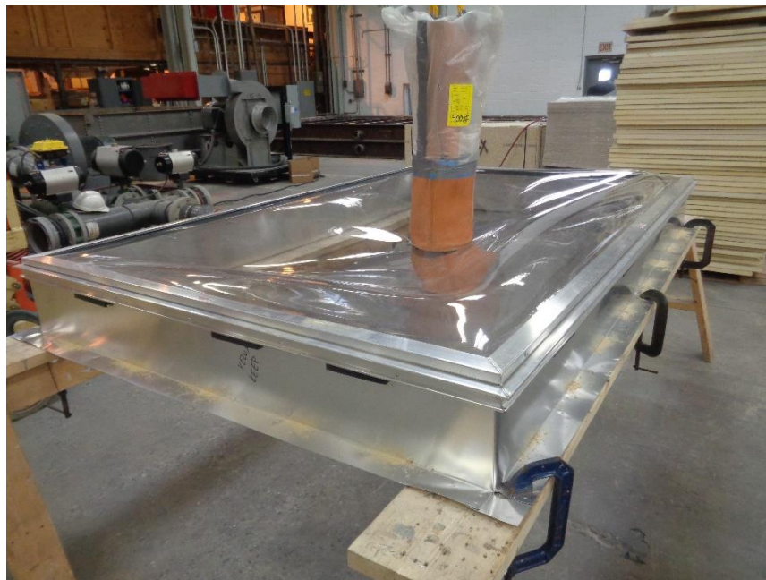
Photo No. 2 View of Tested Specimen with 400 lb Load Applied
