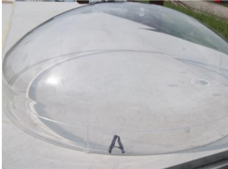
Photo No. 1 Acrylic Dome Represented for Skylight Specimens
