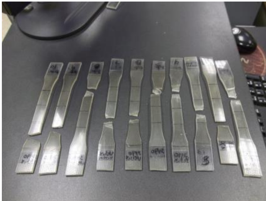
Photo No. 8 Polycarbonate Weathered Tensile Result
