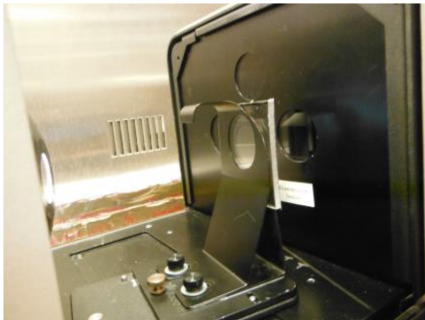
Photo No. 4 Luminance Transmittance Evaluation on Test Specimen
