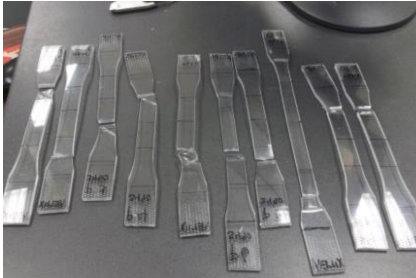
Photo No. 7 Polycarbonate Control Tensile Result
