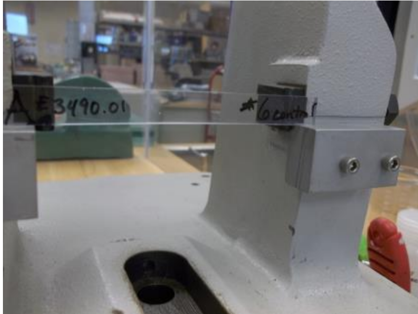
Photo No. 9 Charpy Specimen Loaded for Testing
