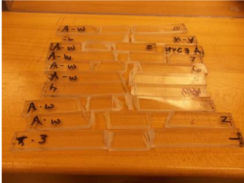
Photo No. 11 Charpy Impact Results for Weathered Acrylic Specimens
