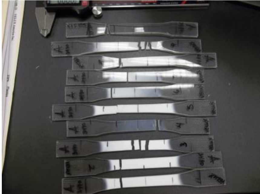
Photo No. 5 Acrylic Control Tensile Samples Result
