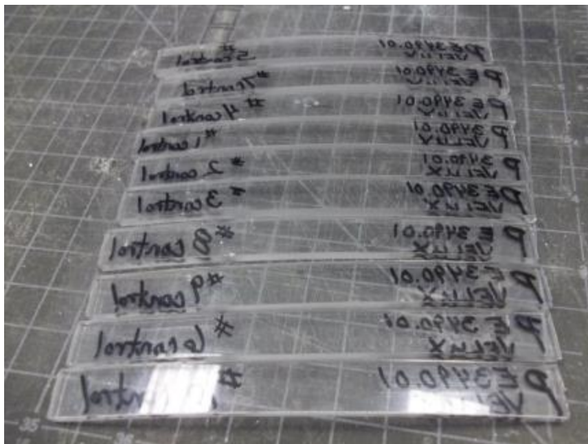
Photo No. 12 Charpy Impact Results for Polycarbonate Control Specimens
