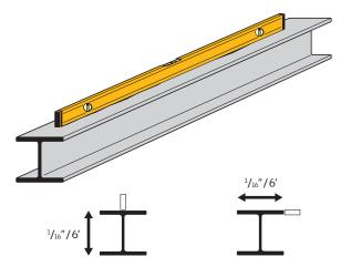
The following standard steel profiles are suited for installation of VELUX modular skylights in Longlight solutions.
