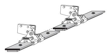
• Connection of flat steel profiles must not collide with clamps
