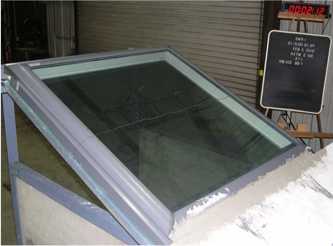
Figure B-1. Skylight prior to Start of Test.
