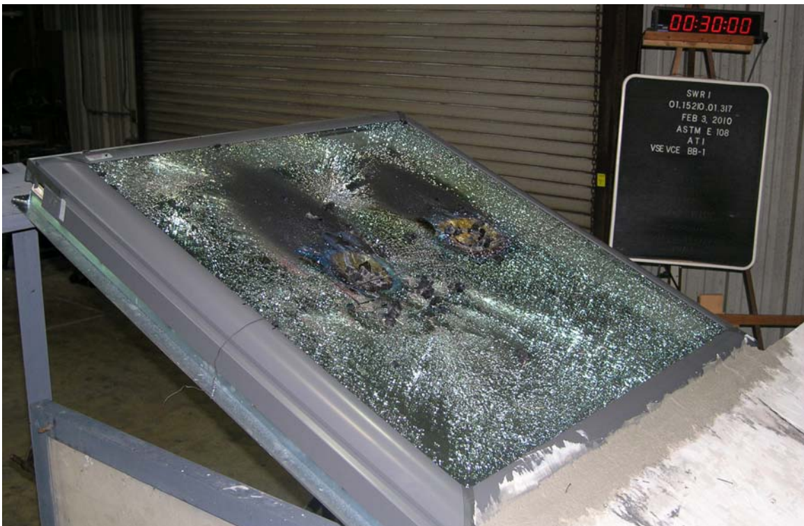
Figure B-4. Condition of Sample at End of Test.
