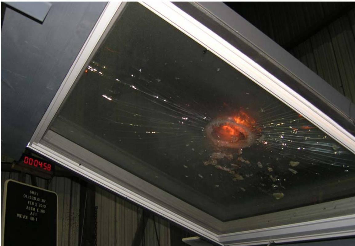
Figure B-2. Pieces of Bottom Layer of Glass Fall onto Screen.
