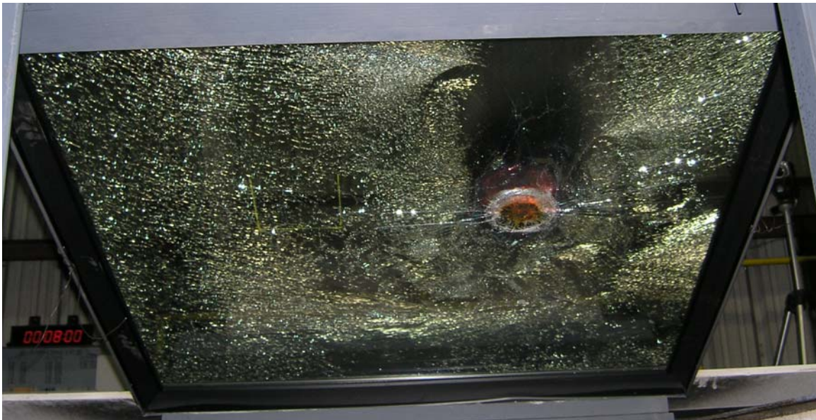
Figure B-3. Shattered Top Layer of Glass.
