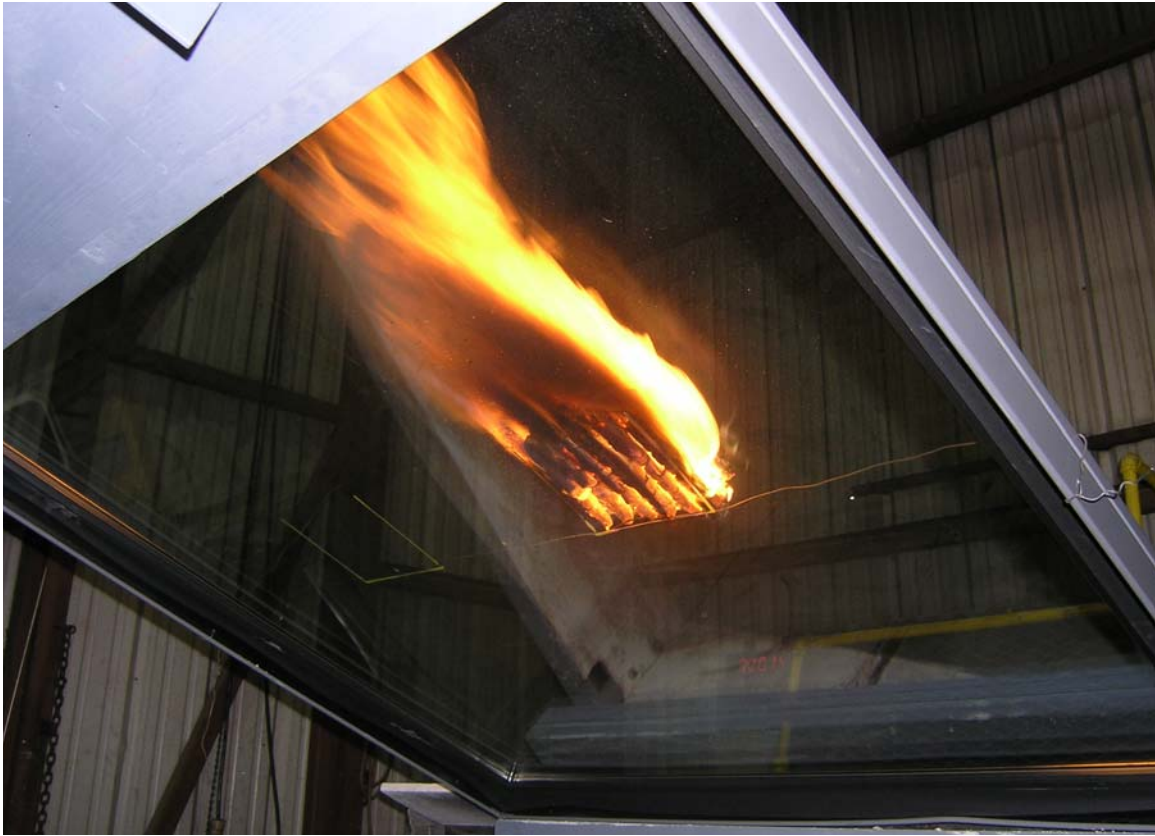
Figure B-1. View of Brand from Underside of Skylight following Brand Placement.
