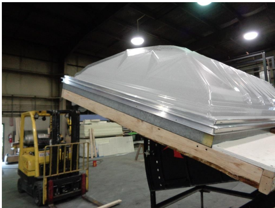
Photo No. 2 IMA Skylight Installed Pre-test
