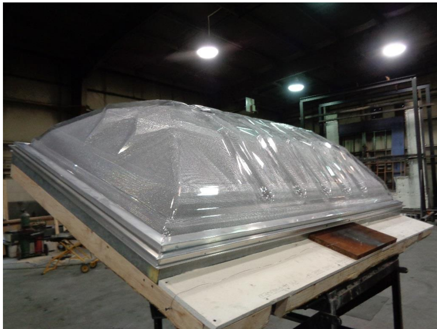
Photo No. 3 Polycarbonate 0.118 Skylight Installed Pre-test
