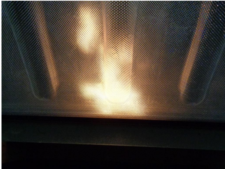
Photo No. 7 Polycarbonate 0.118 Skylight UNDER Deck Burning Brand Test
