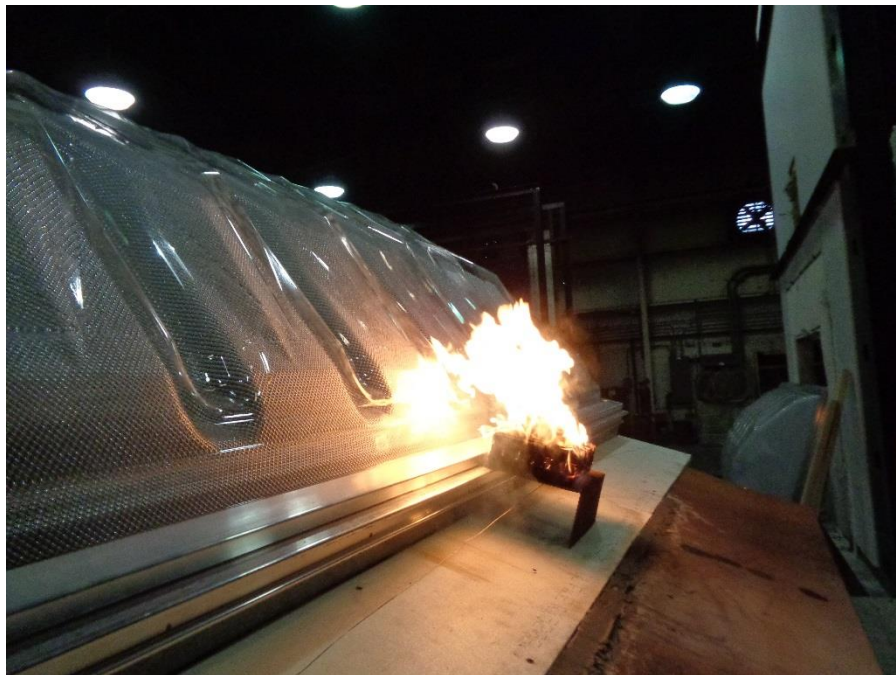
Photo No. 6 Polycarbonate 0.118 in. Skylight During Burning Brand Test
