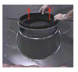
3 Remove the four or five screws in the black intermediate ring. Remove ring by lifting upward. Discard the O-ring gasket only. Keep the screws, as they will be required to reinstall the intermediate ring.
