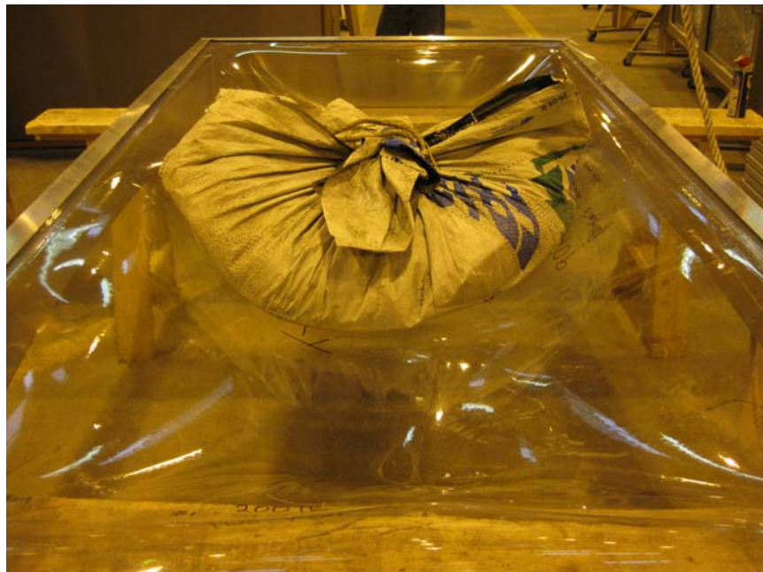
Photo No. 2 CAP-1 (48 x 96) Impactor Fell Through Exterior Glazing Sheet
