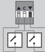
A change-over contact can also be used for running products both up and down but stops are not possible.
