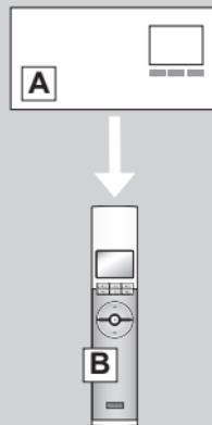
The example shows how to copy the registered products from the interface/repeater unit to a VELUX remote control not yet in operation.
