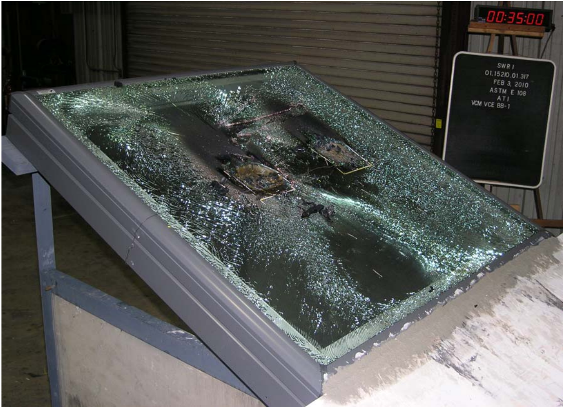
Figure B-3. Condition of Sample at End of Test.
