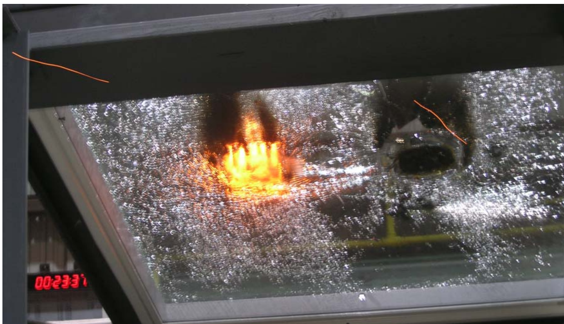
Figure B-2. Underside of Skylight after Placement of Second Brand.
